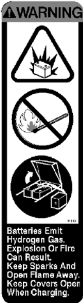
BATTERY CHARGING LABEL - LOCATED IN BATTERY COMPARTMENT AND ON SEAT MOUNTING WELDMENT.
